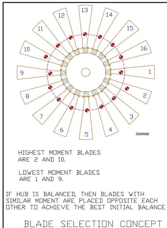
opposite another blade. Jet engine manufacturers can use this method, because they have a large number of blades available, so that it will almost always be possible to find blades of equal static moment. This method cannot be used when rebuilding an engine, since there are only enough blades to fill a single stage.
