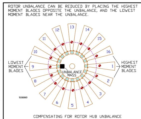
**Conclusions** Gas turbine rotors are among the most difficult items to balance. Assembling the turbine blades in an optimum configuration allows the operator to balance each stage, so that the flexible turbine rotor does not bend when rotated at a high
