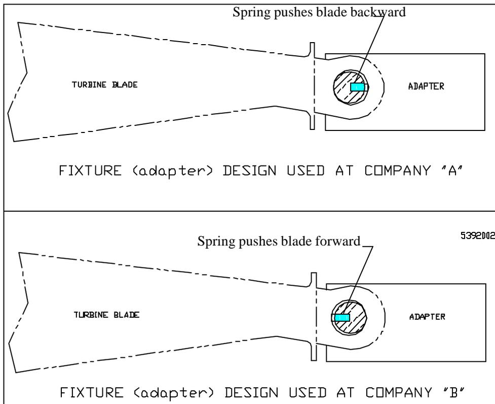
**CASE #5 Another Turbine Blade Fixturing Error** Turbine blades in a jet engine must be sorted by cg moment. Pairs of blades with identical moment are installed in the engine 180 degrees from each other, so that the unbalance is minimized. A jet engine manufacturer was sorting these blades with what he thought was a high precision, yet the engines were badly unbalanced after the blades were installed.
