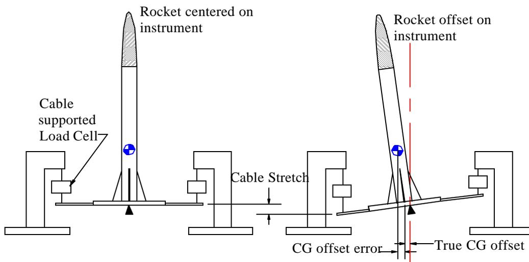
Cable stretch causes the Rocket CG to lean outward, increasing CG offset.
