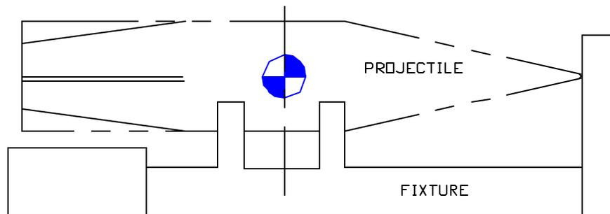
This fixture is designed to contact the nose of the projectile
