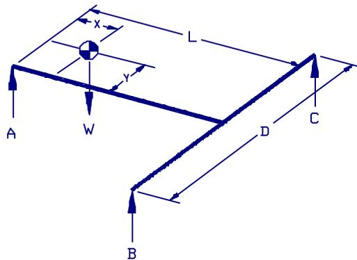
To determine part weight (W) and CG coordinates X and Y, three force transducers are typically used to support a frame which in turn supports the test part.
