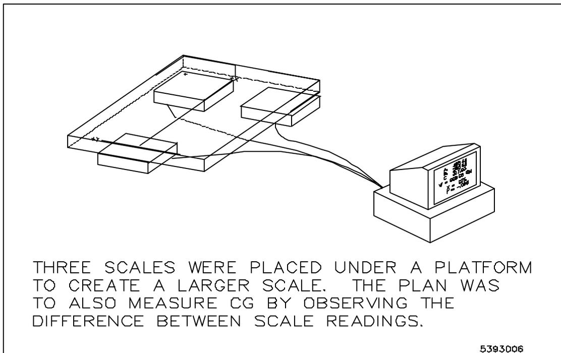
The second step in identifying the problem was to re-assemble the platform and place large test weights on it. The readings changed when the weights were moved. In addition, the total measured weight was larger than it should be. What was wrong??
