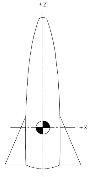
Figure 15 - X, Y and Z are principal axes
