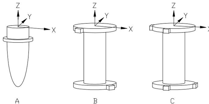
**Figure 17** – Any POI can be simulated by two weights in upper plane and two weights in lower plane
