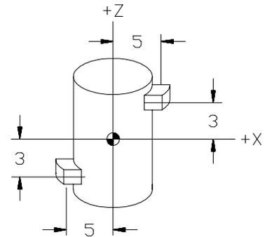
**Figure 20 – Static & dynamic unbalance**
