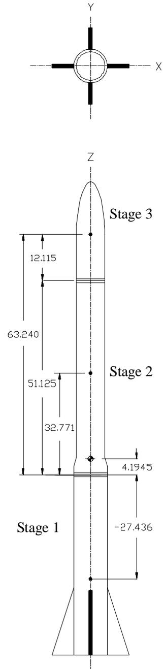
**Figure 8 – CG of Three Stage Rocket**
