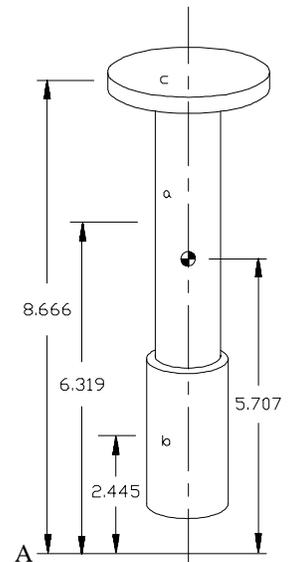
**Figure 7 – CG along a single axis**
