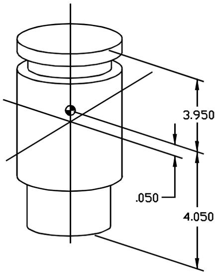
**Figure 1 Center of gravity (and product of inertia) are defined relative to orthogonal axes**
