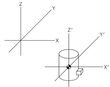
**Figure 22**– POI can be translated to another set of parallel axes
