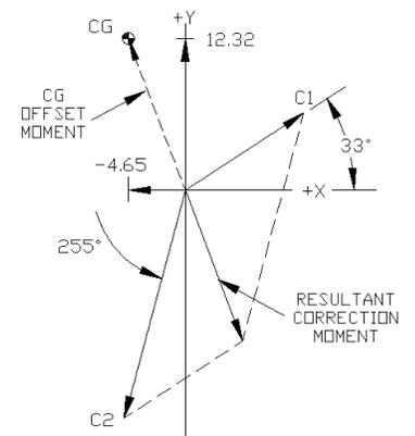
Figure 7 – Static Unbalance
