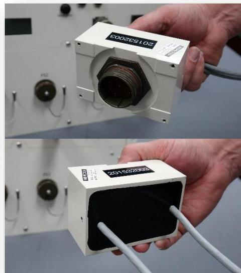
**Failsafe connectors are housed in fully sealed potted assemblies**
