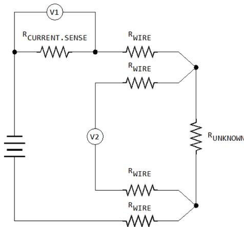
All test circuits use the same fundamental concept. The circuit is constructed of a known precision current sensing resistor in series with the unknown resistor. The processor measures the voltage  $V1$  across the current sense resistor ( $R_{CURRENT.SENSE}$ ) and the voltage  $V2$  across the unknown resistor using a high accuracy differential amplifier. The Ohm's law calculation is
