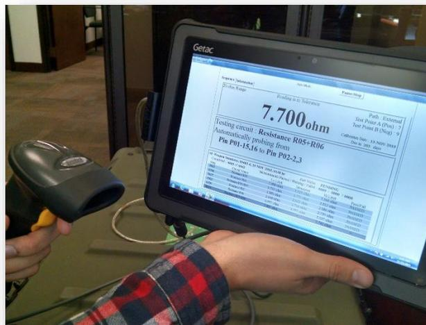
Optional 1D bar code scanner and rugged tablet computer
