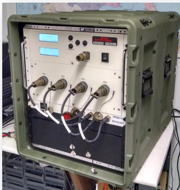
**Model 132-SQB-BTP weapon system circuit tester is a combination 19" rack and bench top unit**
